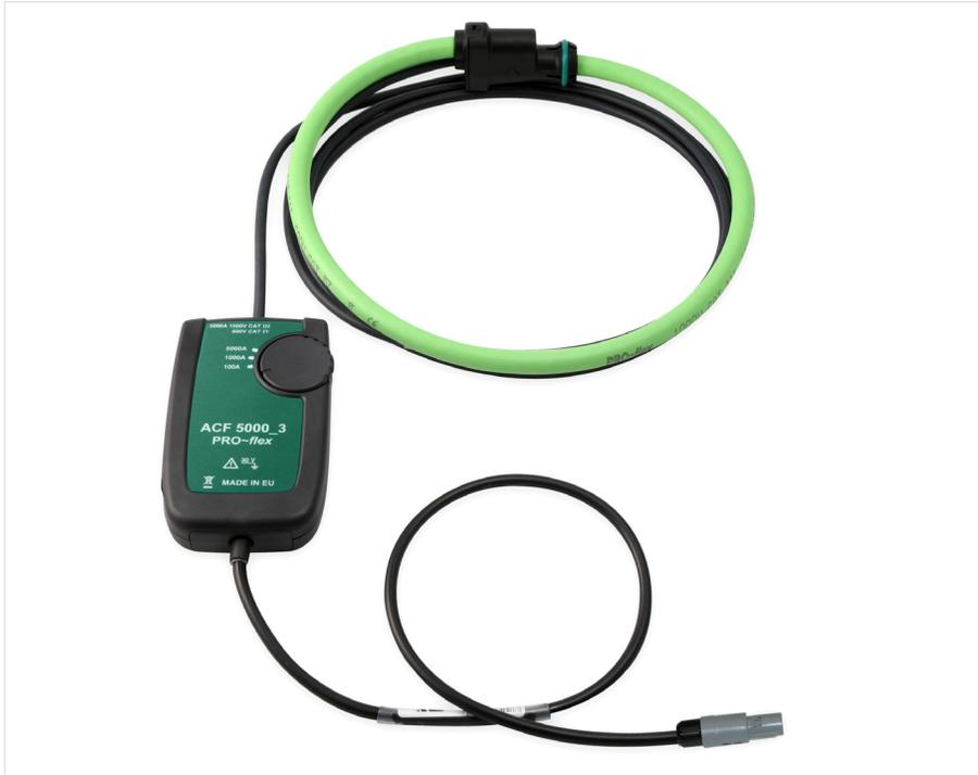
The new PRO-flex ACF 5000\_3 is an AC current Probe utilising the Rogowski principle. It can be used to measure currents up to 5000 Amps from very low frequencies to 10kHz.
